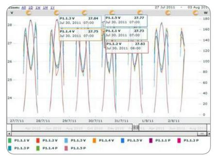
Powerful graphing engine enables analysis of various measures such as voltage, current, power and energy in any scale from module to plant level. Multiple measurements may be displayed on a single graph. Zooming is limited only by the update interval of 5 minutes.
