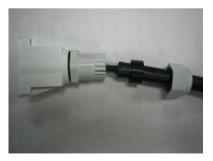
• Twist the gland, attached screws in order to seal the AC gland cover.
