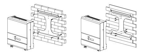
Select the installation location so that the status display can be easily viewed. Choose a strong mounting wall to prevent vibrations while inverter is operating.
