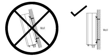
b) Check the upper straps of PV-Inverter and ensure it fits on to the bracket
