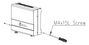
Check the secure mounting of the PV-Inverter by trying to raise it from the bottom. The PV-Inverter should remain firmly attached.
