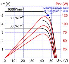
dramatically, inverter is converting the maximum power from panels. When the LCD power reading is significantly changes, Inverter is tracking the power according to the varied sunlight.
