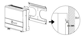
c) Insert safety-lock screws to the bottom leg to secure the inverter
